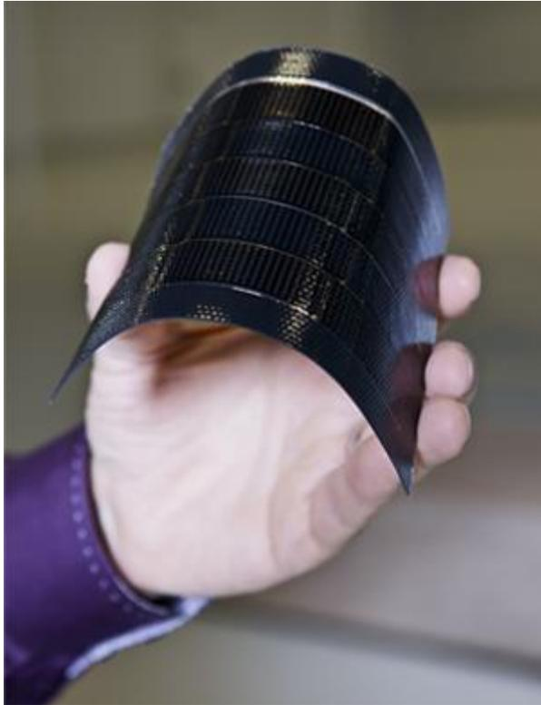
Figure 2 Flexible power: Alta's solar cells can be made into bendable sheets. In this sample, a series of solar cells are encapsulated in a roofing material. Credit: Gabriela Hasbun
