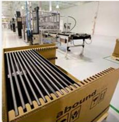
Cheap cells: Abound Solar makes the cadmium-telluride semiconductor for its thin-film solar modules within a single machine, and with no need for wet chemical or etching processes. Credit: Abound Solar
